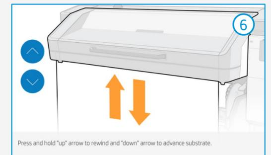
**TIP:** Before cutting the printed job, advance the substrate so that you protect the printed roll when it is unloaded.
